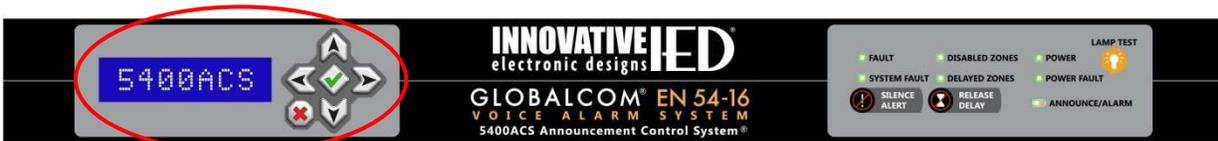
**Figure 2-4: LCD Display & Navigation Buttons**
